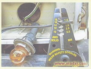
With a wire cutter/stripper remove about 1/4" of the insulation. Wear your safety goggles while doing this (or so it is suggested on this pair of wire strippers from Sears Hardware).
