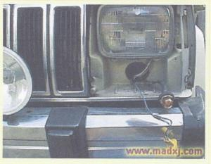
Start with removing the head light bezel, turn signal housing and side marker lens. Gently pull the wires out for the turn signal and side marker.
