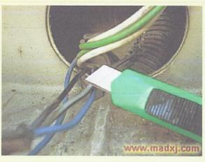
With a box cutter (or similar) make two cuts into the *insulation only* of the gray (with black tracer) wire (driver's side) or brown wire (passenger's side). Don't cut any of the copper strands. Cut the insulation all around the wire's circumference.
