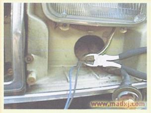
Then clip the *side marker's* ground wire which is the black one. Clip it far enough back so you won't have to extend it later. The side marker wires need to be long enough to reach up into the side marker lens.
